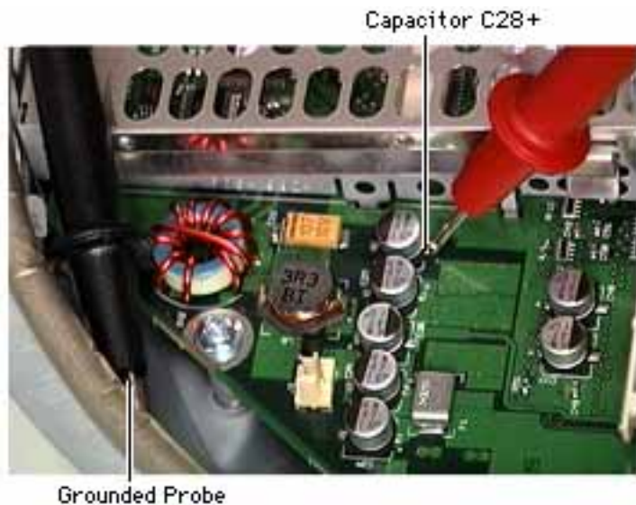
Testing for Power at the Logic Board
