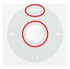
2. When the Apple icon appears, attempt to put the iPod into Disk Mode by immediately and simultaneously pressing and holding the Play and Center buttons,
